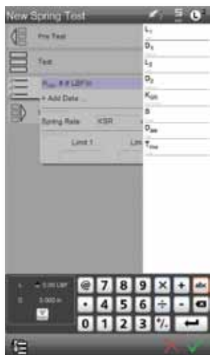
The Data section is used to specify which results are reported at the completion of a test. This section is used to format how results will be displayed. Additionally, this section is used to establish tolerance limits for each result.
