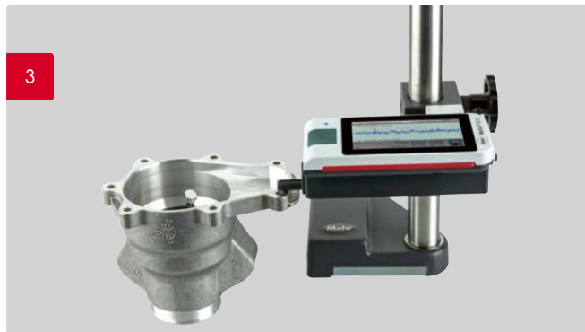
3. Roughness measurement with measuring stand ST-D
