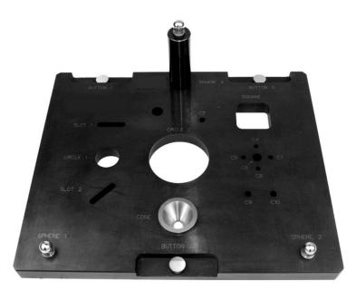
Our CMM Calibration Artifact is designed for use as an Intermediate Check with Coordinate Measuring Machines (CMMs) and includes an ISO-17025 Accredited Certification.
