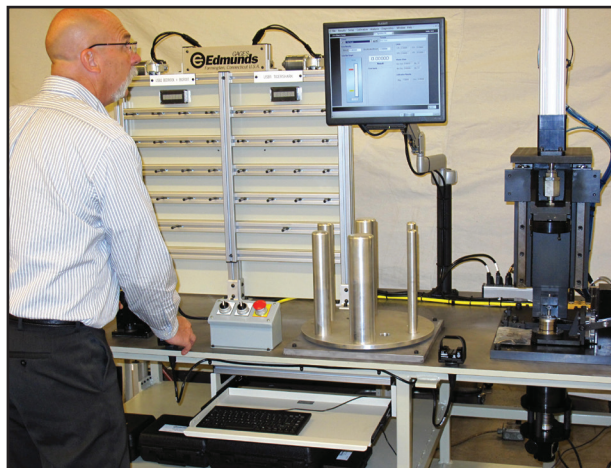
Pick-to-light select fit stations.
