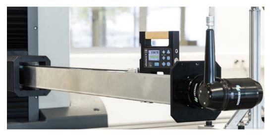
Machining Industry -Inclination control of the position of a measuring arm on a large 3D coordinate measuring machine With the help of the TESA CLINOBEVEL 3, the angular deviation in the respective position of the arm can be easily determined. Results are then used for correction / compensation of the measuring system.
