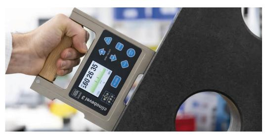
High precision control of a granite plate. The big measuring range of  $\pm 60^{\circ}$  enables also to fulfil new measuring applications (image above).
