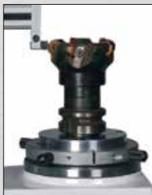
Checking of a Runout
