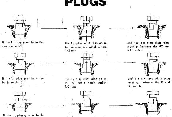
the L, plug must also go in to the minimum notch within 1/2 turn
