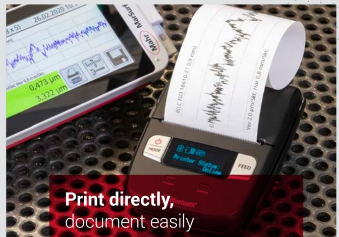
The new mobile roughness measuring instrument MarSurf M 310, has easy operation and a robust design.
