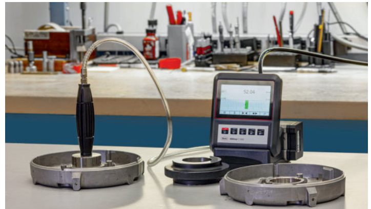
Stand alone air gaging for bore diameter
