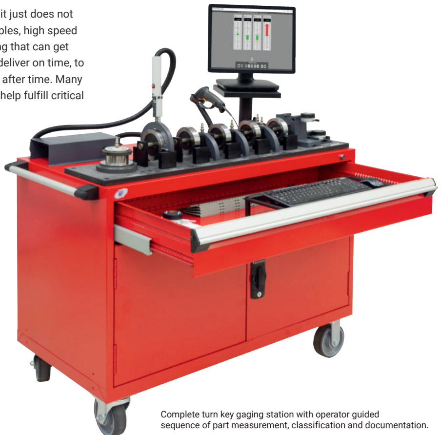
Stand alone air gaging for bore diameter
