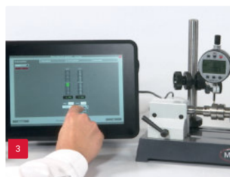
Radial run out measurement with dial indicator
