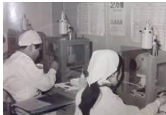
Figure 29 Inspecting gauge blocks (1966)
