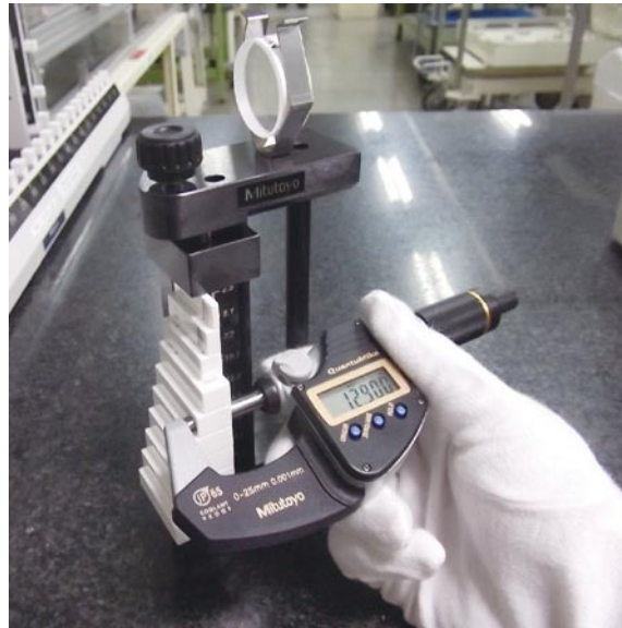
Figure 47 Micrometer-check gauge block holder (developed in 2002)
