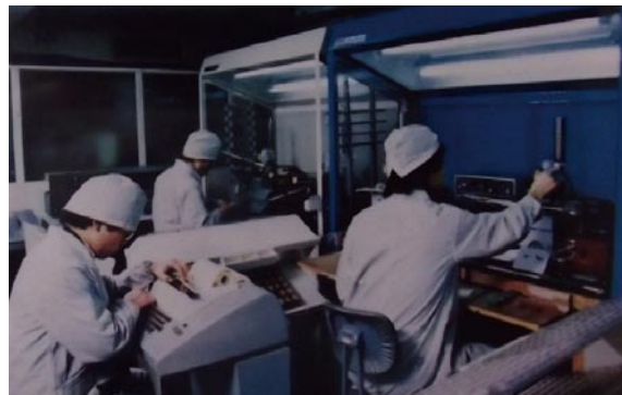
Figure 31 Calibrating gauge blocks with the original automatic calibration tester
