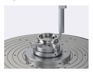
The surface roughness of bearings requires high-precision measurement since it has direct impact on the coefficient of friction. A single ROUNDTRACER EXTREME can not only efficiently measure roundness, but also surface roughness with high accuracy.
