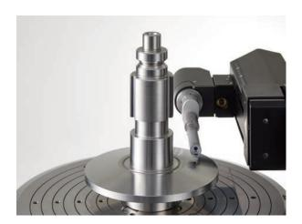
Pulley based CVTs are components of automotive continuously variable transmissions that contribute to fuel efficiency and smooth travel. Provides measurement of surface roughness of the tapered portion, roundness, and contour. This previously required multiple measuring instruments and setup but can now be efficiently conducted using a single measuring machine.
