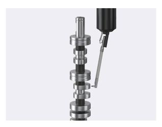
Camshafts require high-precision measurement because they control the opening and closing of inlet/outlet valves that improve the combustion efficiency of engines. Measurement of cam shape, surface roughness, and roundness, which previously required multiple measuring instruments and setup, can now be efficiently conducted using a single measuring machine.
