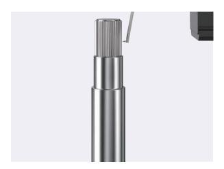
The rotating X-axis tracking measurement function enables all-round measurement and assessment\* of splines exceeding the measuring range of the detector.
