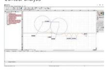
Provides not only a range of basic commands for analyzing points (10 types), lines (6 types), and circles (6 types), but also a wide variety of commands to calculate angles formed by a combination of items, pitches, distances, etc., contour matching function, and design value generation function as standard features.
