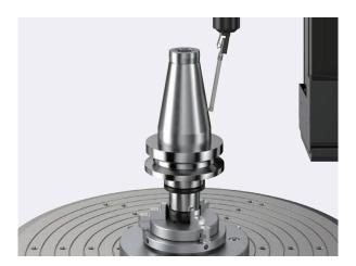
The tapered portion of tool holders requires high-precision measurement since it needs to pair with the main axis of machine tools. High-precision positioning by the newly developed centering element and Z axis slider enables highly reproducible measurements.
