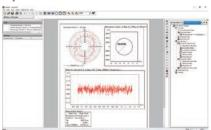
Allows for layout of contour, surface roughness, and/or roundness measurement results and graphics on a single sheet of paper by using simple operations. Furthermore, support for pasting from specified saved files allows results to be pasted from multiple files.
