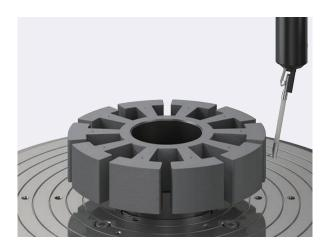
Motor cores, which are the base of motor assemblies, require high machining accuracy. ROUNDTRACER EXTREME allows for efficient, high-precision workpiece setup for rectilinear contour measurement at multiple points.
