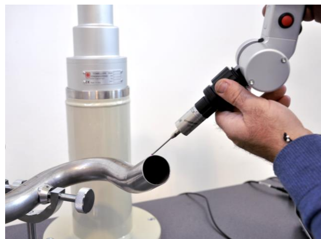
Pipe measurement by touch probe
