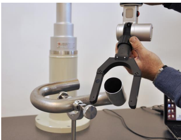
Pipe measurement by laser fork
