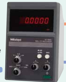
Digital differential type Mu-Checker No. 519-562A (with Digimatic output) P15
