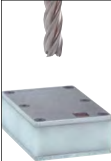
Slowly lower cutting tool toward Tool Setter
