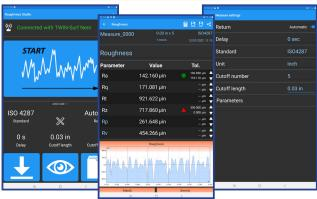
With the standard Roughness Studio APP, the instrument can be connected to an Android or Windows device and allows you to download measurement data in real time or at a later time from the internal memory of the roughness tester.
