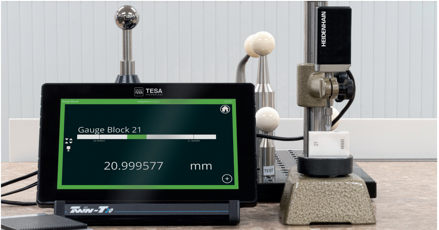
Checking of ceramic gauge block
