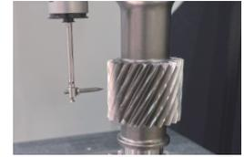
Measuring example with a stylus for contour measuring instruments. Narrow roots can be measured.
