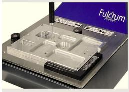
Magnetic fixture templates allow you to quickly fixture your part, making sure that all points are taken accurately.
