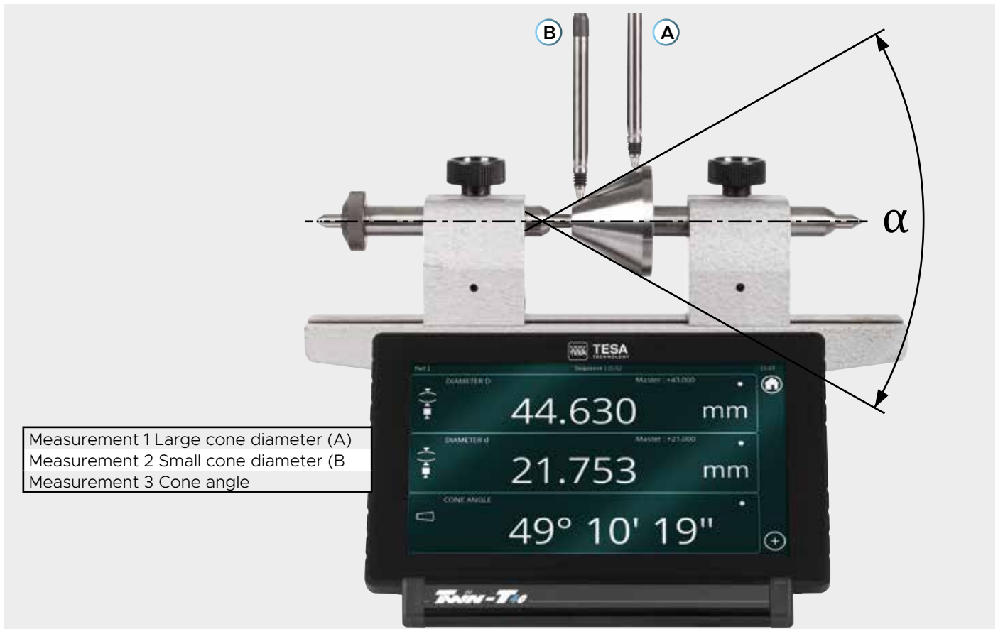
Measurement of cone angle using trigonometric functions.
