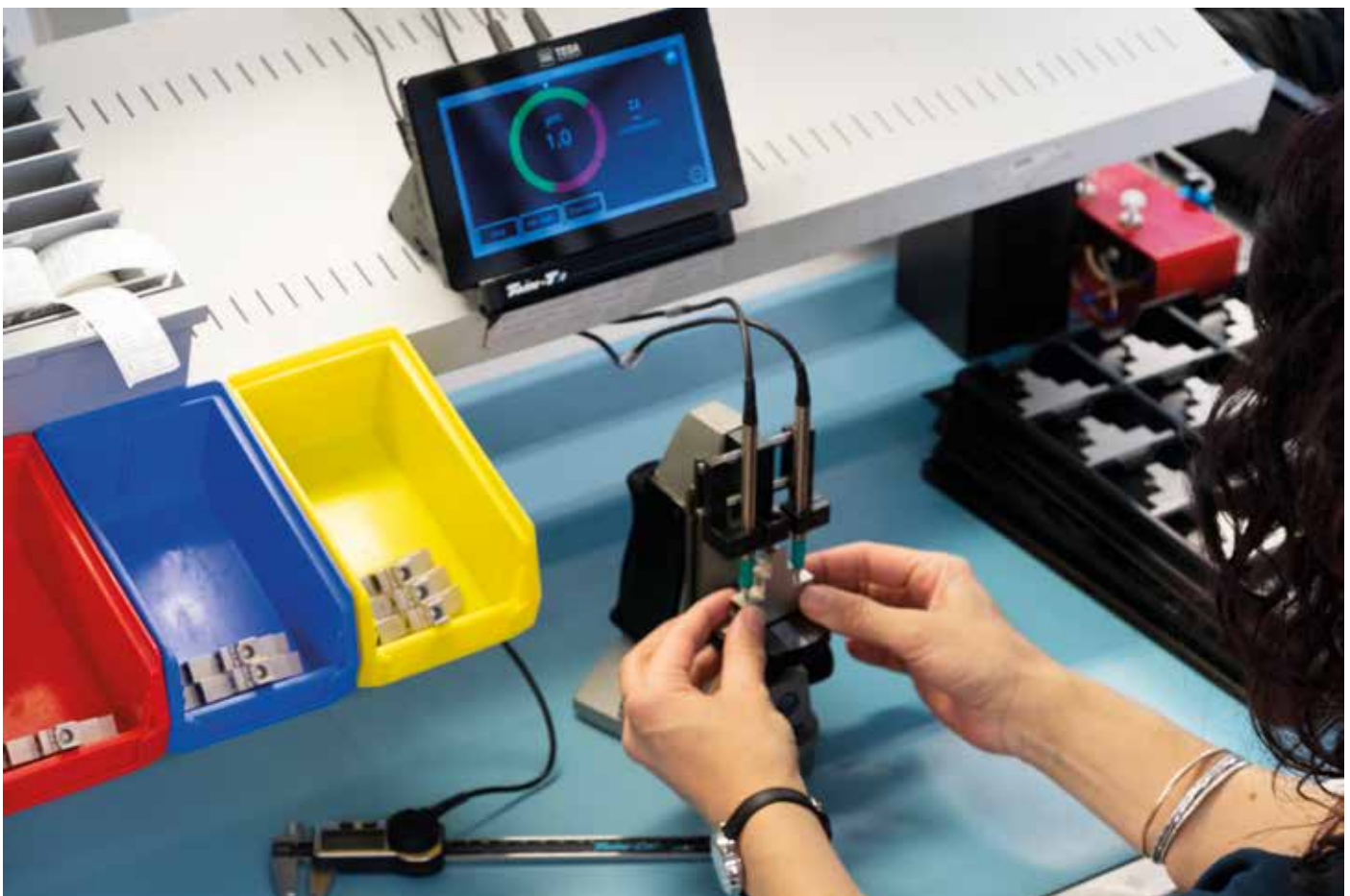
Part classification: the operator classifies the parts in the bin in the same color as the screen outline.
