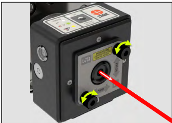
Step 5 - Turn on the T-1297 Target and go to Step 2, where it will connect to Plane6. Move the T-1297 to the far end of the straight edge and adjust the L-703SP's pitch/yaw angular knobs until the readout is within 5000 \mu\text{in} . (130 \mu\text{m} ).
