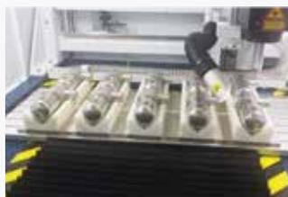
*Parts are nested in machined plastic blocks that are affixed to Loc-N-Load™ plates. To make the process even more visual, fixtures are identified by their numbers and etched with associated part model numbers.*
