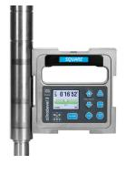
The magnetic measuring faces stabilise the instrument and reduce any influence on the measurement.
