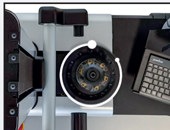
Automatic spindle rotation and tool edge measurement
