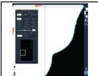
Automatic DXF acquisition of cutting tool profile
