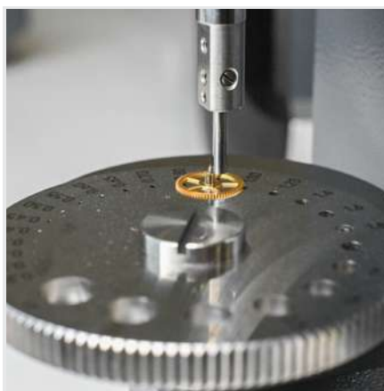
Measurement of small parts with PS15BV+ and rotation 25 holes support
