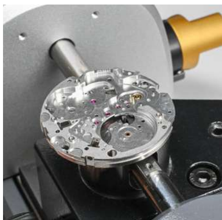
Internal measurement in 3 – points
