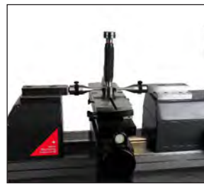
Checking of thread plug gages, from m100 upwards (TA-SU-313, TEL6, 3P/0.17-3.2/S6.5)
