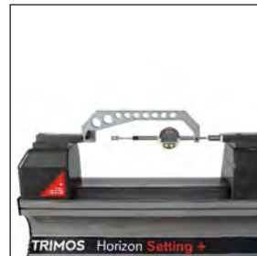
Checking of dial indicators and comparators (TA-IH-301)
