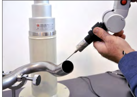
Pipe measurement with touch probe
