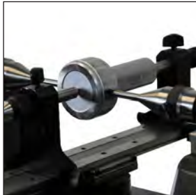
Checking of plug gages and pin gages, Max. ø 100mm/4", length 280mm/11" (TULM6/L0.5, LABC15)
