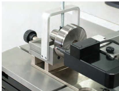
Checking of taper thread plug gages
