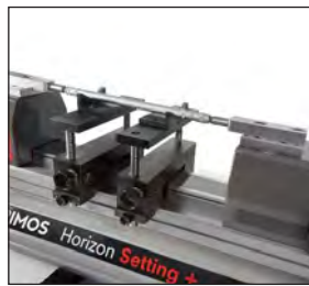
Setting of 2 point internal measuring equipment (TELMA7)
