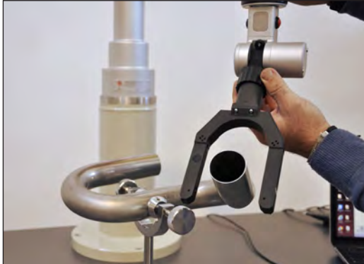
Pipe measurement with laser fork
