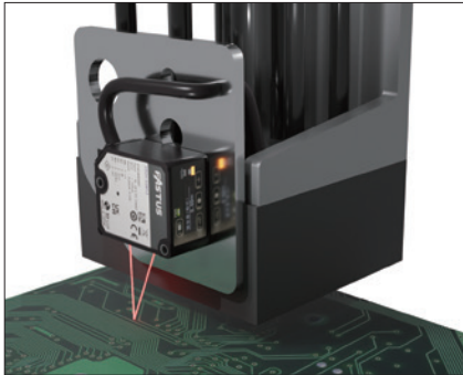
Height Measurement of Mounted Components
