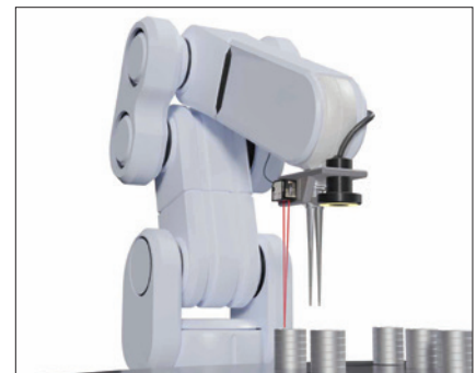
Stacked Bearing Height Measurement
