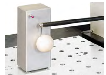
2-sphere calibration standard
